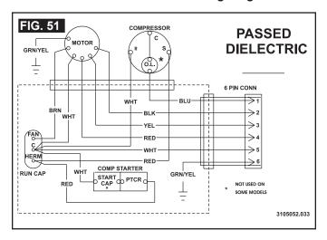
5. 541915 & 541916 Unit Wiring Diagram
