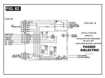
4. 3313189.064 & 3313189.072 LCD SZ Electronic Control Kit Wiring Diagram Cool/Furnace/HP
