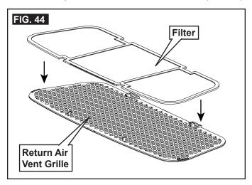
6. Install return air vent grille into the ADB. Slide return air vent grille tab into slot in ADB and rotate up and snap in place. See (FIG. 45).
