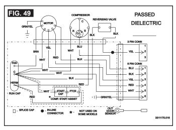
3. 459196 & B59196 Unit Wiring Diagram
