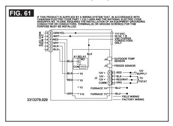
3. 3313189.049 & 3313189.056 LCD SZ Electronic Control Kit Wiring Diagram Cool/Furnace/HS
